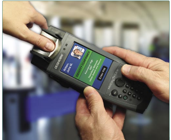
DAP's Guard System features a 500 dpi fingerprint reader for easy biometric authentication.
