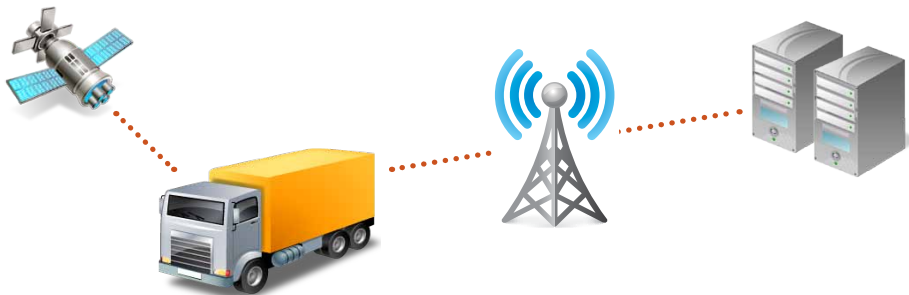
A single DAP tablet replaces multiple systems by gathering and relaying real-time location and telemetry data to database servers via a Wireless Wide Area Network (WWAN).
